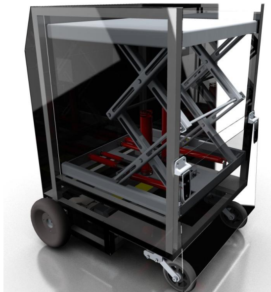
Figure 9: Actual state of the ECB with platform and adjusted Casters [17]
